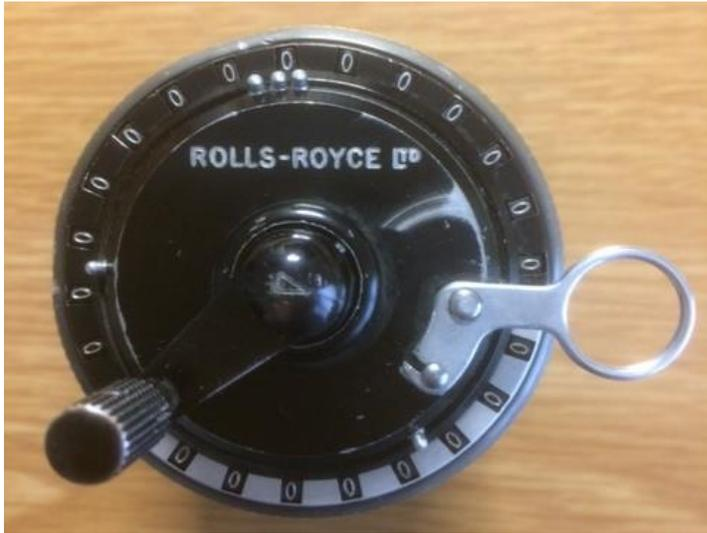
Top view showing the new clearing ring lever.
